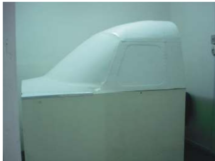
Cock pit cover of simulator to give a realistic feel. Cockpit cover will later be painted to represent aircraft livery 5Y ACE.
